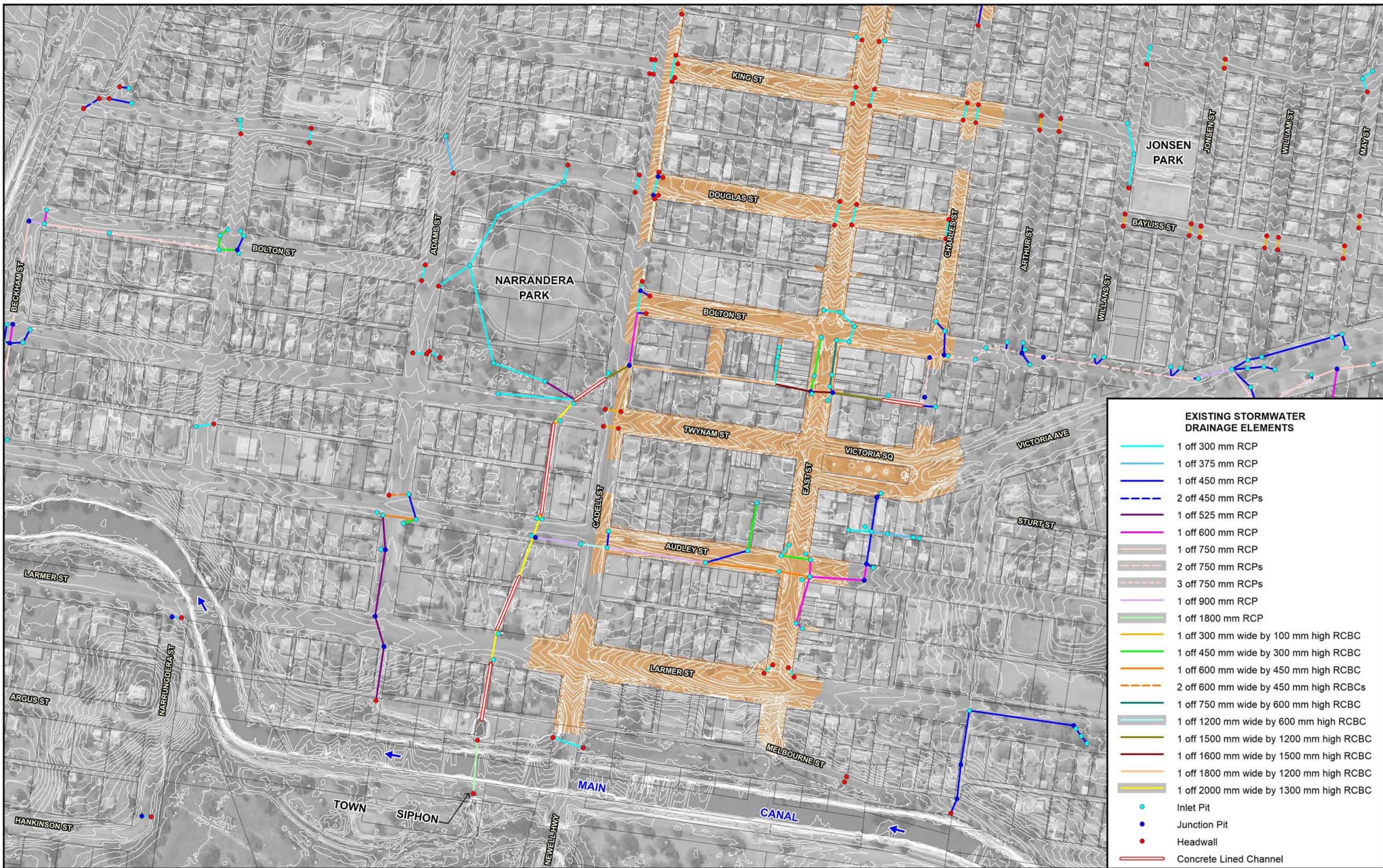
Figure 1 LAYOUT OF EXISTING DRAINAGE SYSTEM IN VICINITY OF NARRANDERA CBD
