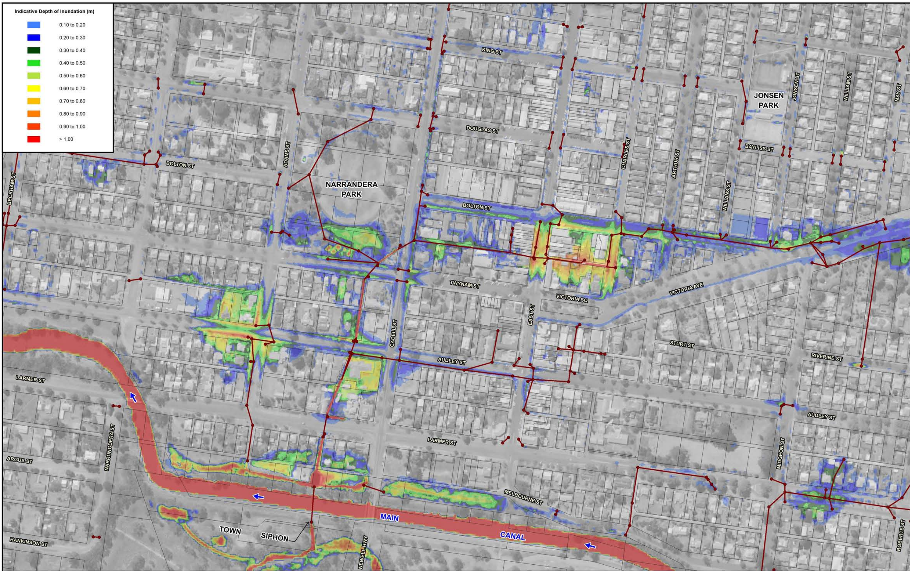
Figure 4 INDICATIVE EXTENT AND DEPTH OF INUNDATION PRESENT DAY CONDITIONS - 1% AEP
